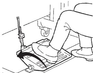
4. Press the machine treadle with toes.
